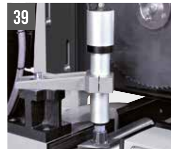
TIGER 352 MA/COBRA 352 MA Morsa verticale pneumatica
